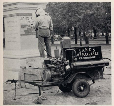
For the dealer whose inscription volume does not warrant purchasing a Model T-33, Lindsay builds the popular Model 15 Air Compressor which costs only \$460 including automatic unloading. This compact, rugged machine has power for blowing 1½" inscription letters in granite, using electric furnace abrasive, in less than two minutes each.
