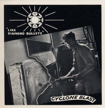
Aluminum Oxide and Silicon Carbide Abrasives
