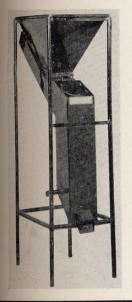
A necessity for clean Shot and Abrasive so as to produce whiter panels and remove dust from Abrasive to obtain faster cut.
