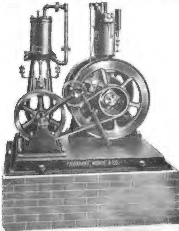
FAIRBANKS-MORSE VERTICAL ENGINE AND AIR COMPRESSOR. For a number of years stone workers have been interested in pneumatic machinery to be used in connection with stone dressing and carving, and in many large establishments, where considerable power is required, stone carving has been extensively carried on by the use of pneumatic chipping hammers. As these hammers are operated by compressed air some power plant is required to operate the compressor which supplies the air to the tools. There has been very little difficulty in supplying the larger establishments with a combined engine and air compressor, but generally these combinations were not made in sizes smaller than 12 H-P, and a plant of this size would operate from fifteen to twenty hammers, which is very much larger than would be required in the majority of monumental works. As the majority of the smaller yards would only require two or three hammers a very desirable combination would be a smaller gasoline engine and air com-
