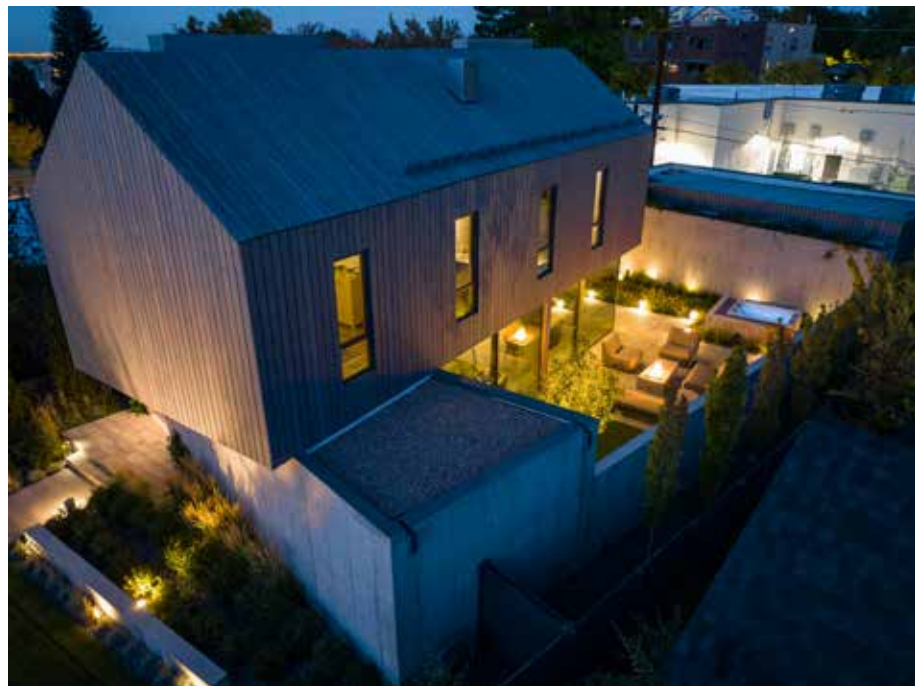
The upper volume of the modern single-family residence designed by Meridian 105 Architecture sits at an angle, diagonally offset from the ground floor in order to increase natural light in the interior. It's fully clad in light-gray Accoya, a chemically-modified acetylated pine product imported from Scandinavia.
