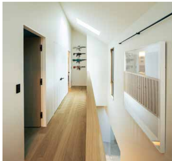
The stair rail detailing is Meridian 105 architect Daniel Lipscomb's design, and was executed by a woodworker on site. The rail is made of two solid wood pieces and includes a carved-out, LED-lit channel for the hand to follow. LEFT: A piece from artist Éric Nado's Typewriter Guns series, in which the artist meticulously sculpts objects out of recycled typewriter parts as a commentary on gun culture, is installed at the end of the upstairs hallway.
