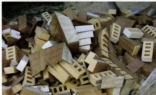
Above: The team salvaged brick from old buildings to match the dimensions of the brick used in the home’s original construction. Because it was going to be painted, it didn’t matter what color it was.
