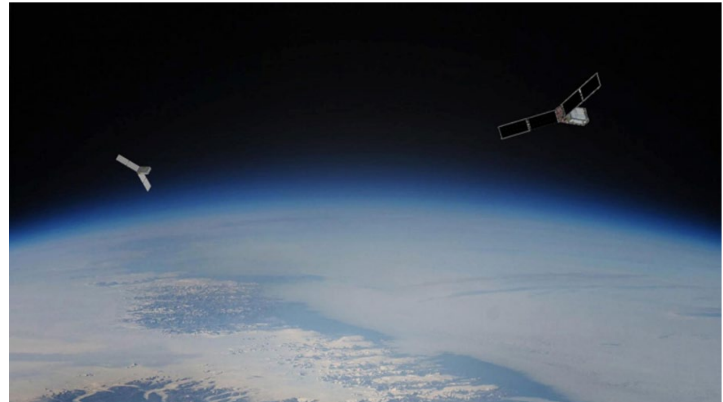
The PREFIRE mission will send two CubeSats into space to study how much heat the planet absorbs and emits from its polar regions. (Source: NASA Jet Propulsion Laboratory / NASA/JPL-Caltech, Public domain)
