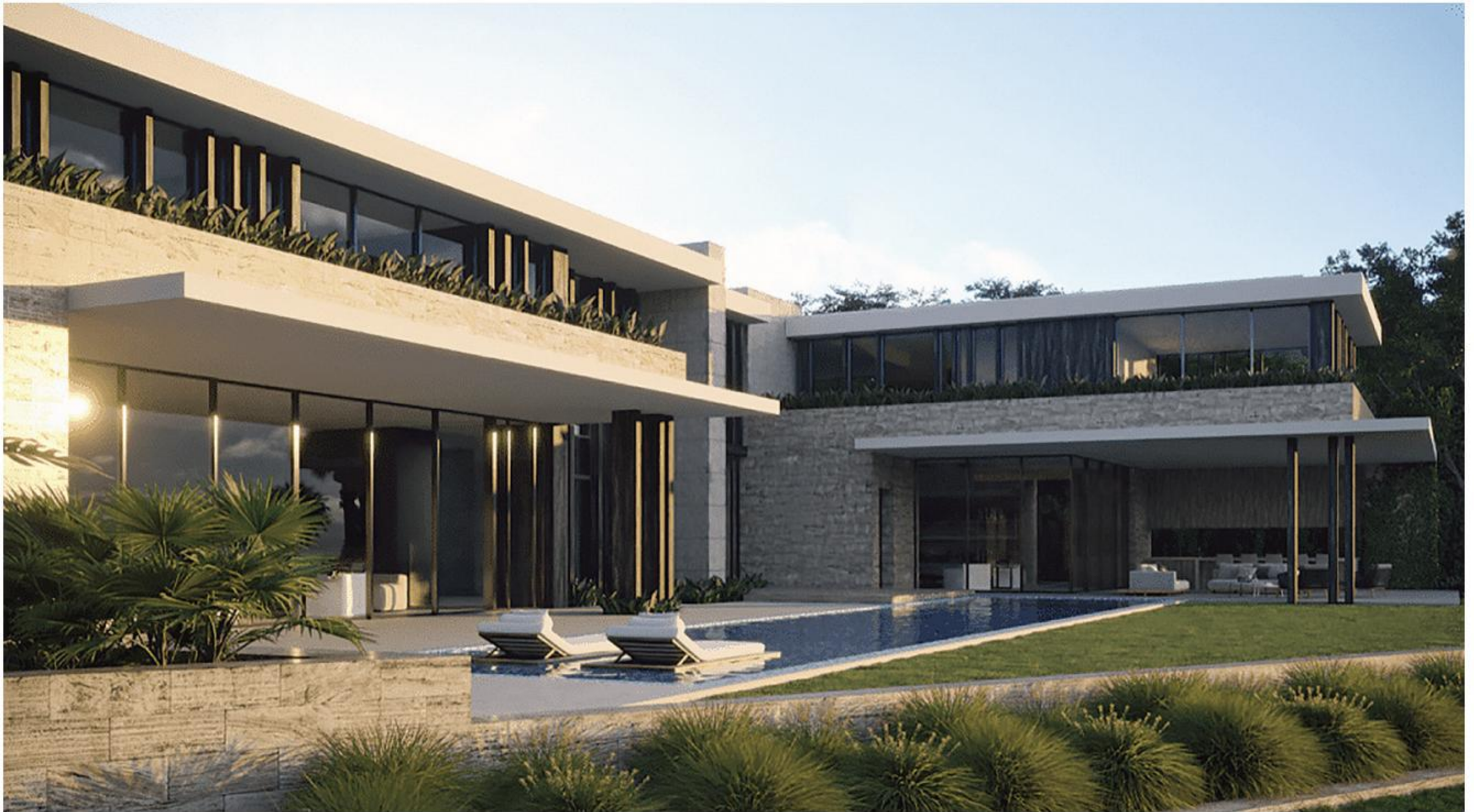
Panther National homes will feature deep, overhanging eyebrows and vertical brise soleil to reduce direct sun naturally, making them more energy efficient.
