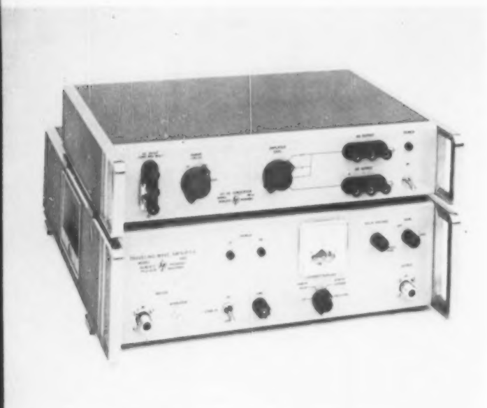
8—Electronic enclosure system, Hewlett-Packard Co.
