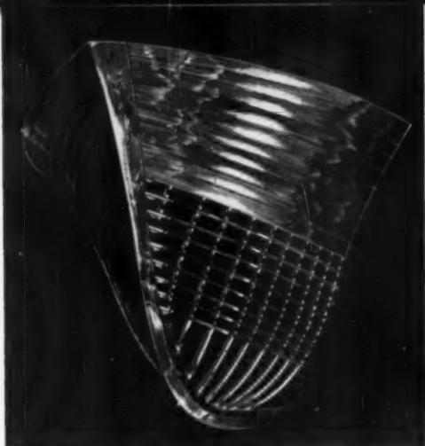
Avro's planked aluminum hull
