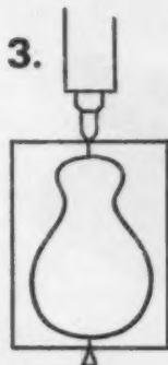
3. Air forces tube against mold sides
