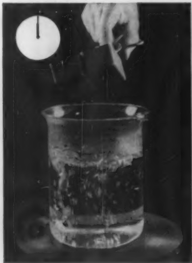
Boiling water provides a positive test for two deep drawn* vinyl-clad parts. Neither special care in forming, nor post curing has been used to prepare either part.
