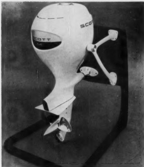
McCulloch Scott 120 horsepower, supercharged fuel-injection outboard motor takes up no more space than conventional 50 horsepower engine. Homogeneous form of experimental fiberglass housing is achieved through development of single unified surface. Reinecke Associates, designers.
