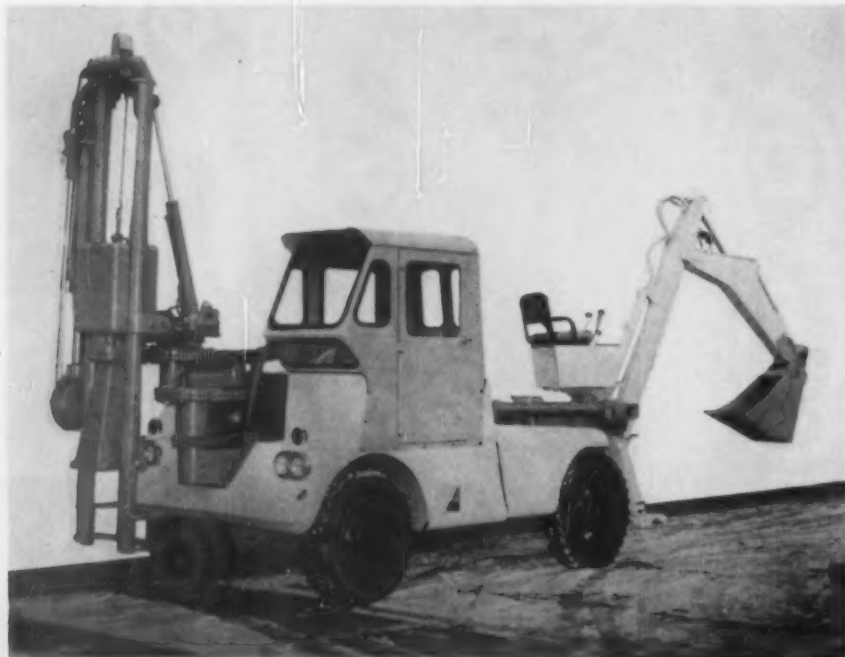
Ottawa Commando is a basic prime mover with a dozen "uni-tools" that convert it to power crane, aerial tower, fork lift, tractor, bulldozer, or snow plow. Attached to the front end, above, is a hydra-hammer to break concrete and tamp fill. The rear end carries a hydraulic backhoe. A shuttle transmission with split torque drive arrangement permits Commando's operation as a truck or tractor.
