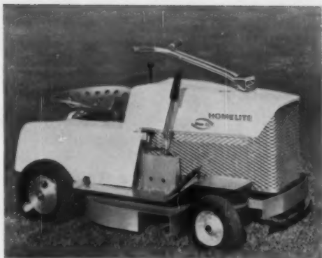
Homelite mower car designed to "drive like a car," has three-speed automatic transmission plus reverse and neutral. Needs no clutch. Automatic braking and down-hill braking. Lever adjusts cutting height to five positions. Aluminum grille, fiberglass body. Lippincott and Margulies, designers. $450.
