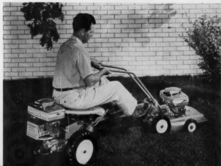
Outboard Marine's Lawn-Boy Loafer has four forward speeds, reverse and neutral. Quietlite engine floats on three rubber shock mounts that isolate vibration and is sealed in a thickly insulated fiberglass soundtrap bonnet to reduce noise. Brooks Stevens, designer. $114.50.
