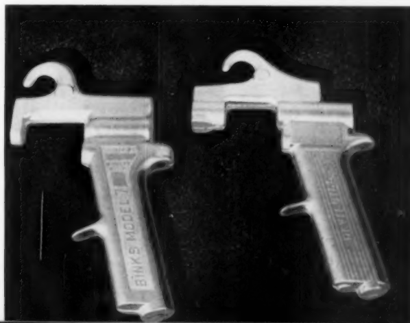
7. Solid aluminum parts can be formed by forging; parts can vary in weight from few ounces to thousands of pounds. Photo: Alcoa.
