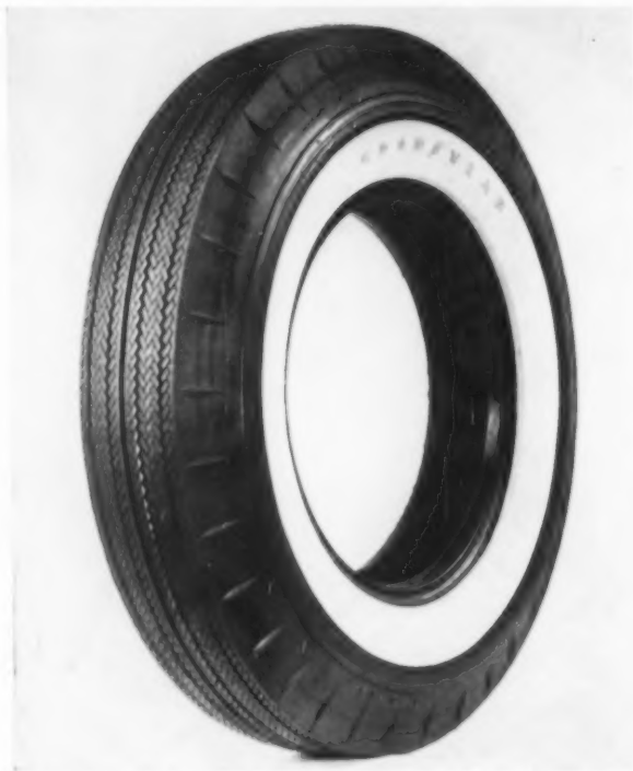
Original equipment tire is type supplied by Detroit on standard passenger cars and its pattern is as crisply defined as the factory-fresh chrome and steel body under which it will ride. Passenger car tires involve more compromises than any other type of tire because they will be used interchangeably on all four wheels. The lateral cuts required for rear-wheel traction and circumferential grooves required for front-wheel steering end up as diagonals—herringbone cuts, zigzag grooves.
