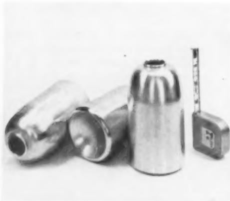
4. Aerosol cans formed by impact extrusion have no seams or welds. Photo: Alcoa.
