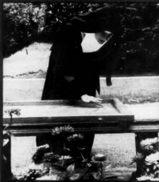
Drying the gum screen. "The glue formula is 50 per cent LaPage's glue, 40 per cent water, 8 per cent white vinegar, and 2 percent glycerin."
