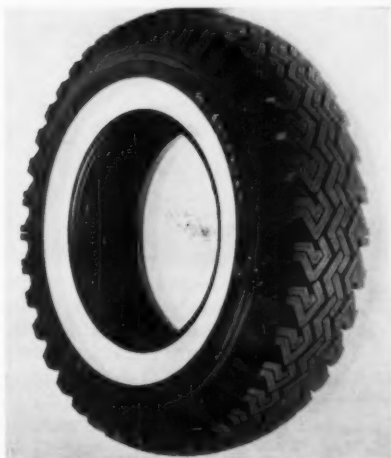
The 1958 Suburbanite is the first designed by the Wilson office. Traction lugs have been grouped into continuous zig-zag bands which give the tire an aggressive look. They also extend its life and make it more versatile. Placing the lugs closer together gives their vulnerable tips support from neighboring lugs, so the tire lasts longer; grouping them in bands makes for a quieter ride on clear roads. Mud and snow traction is provided by numerous acute angles and sharp edges of lugs within the circumferential bands, and by lateral pattern of the lugs at the sidewall.
