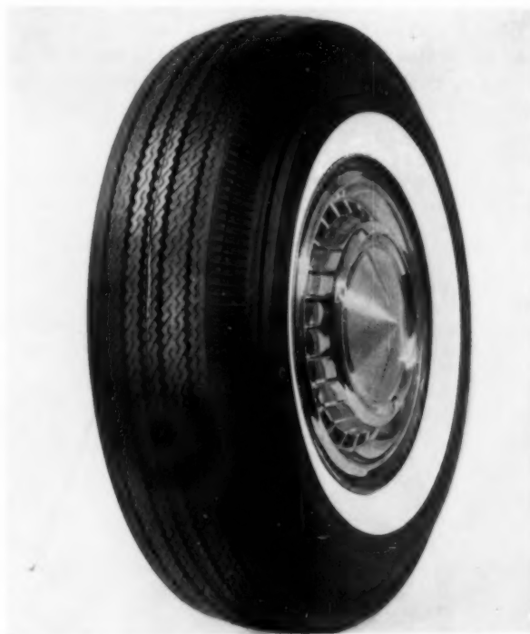
Premium passenger tire uses essentially the same design elements as original equipment tire, but its tread is deeper for longer wear (all tires have linking tie-bars beneath the incisions to lengthen tire life). Pattern on premium tire is more subtle; traction cuts are not connected and tire looks softer, quieter riding. Sidewall, one area of tire in which design gets a free hand (sidewall does not affect performance) here is patterned with close-spaced radials and a band of diamonds.
