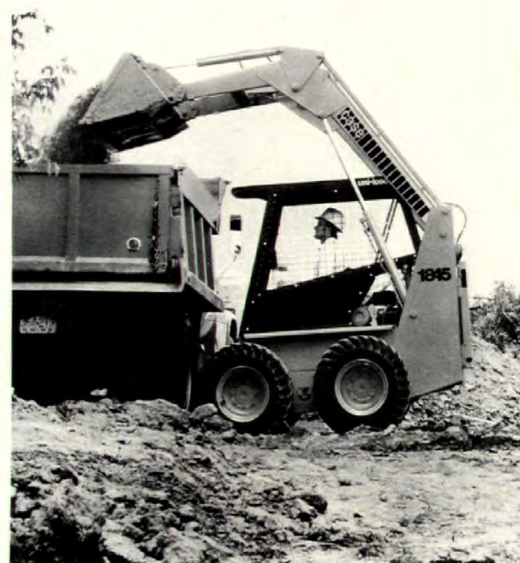
Compact "Uni-Loader Model 1845" features hydrostatic four-wheel drive. Engineered for high-production loading and material handling, unit has the ability to spin-turn in its own length. J. I. Case, Racine, Wisc. CIRCLE 258 ON READER SERVICE CARD
