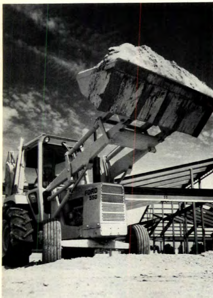
Tractor/loader/backhoe, "Model 550," is available with a gasoline or diesel three-cylinder engine. Vehicle has a breakout force of 8000 lbs and a full-height lift capacity of 4700 lbs. Ford Tractor, Troy, Mich. CIRCLE 254 ON READER SERVICE CARD
