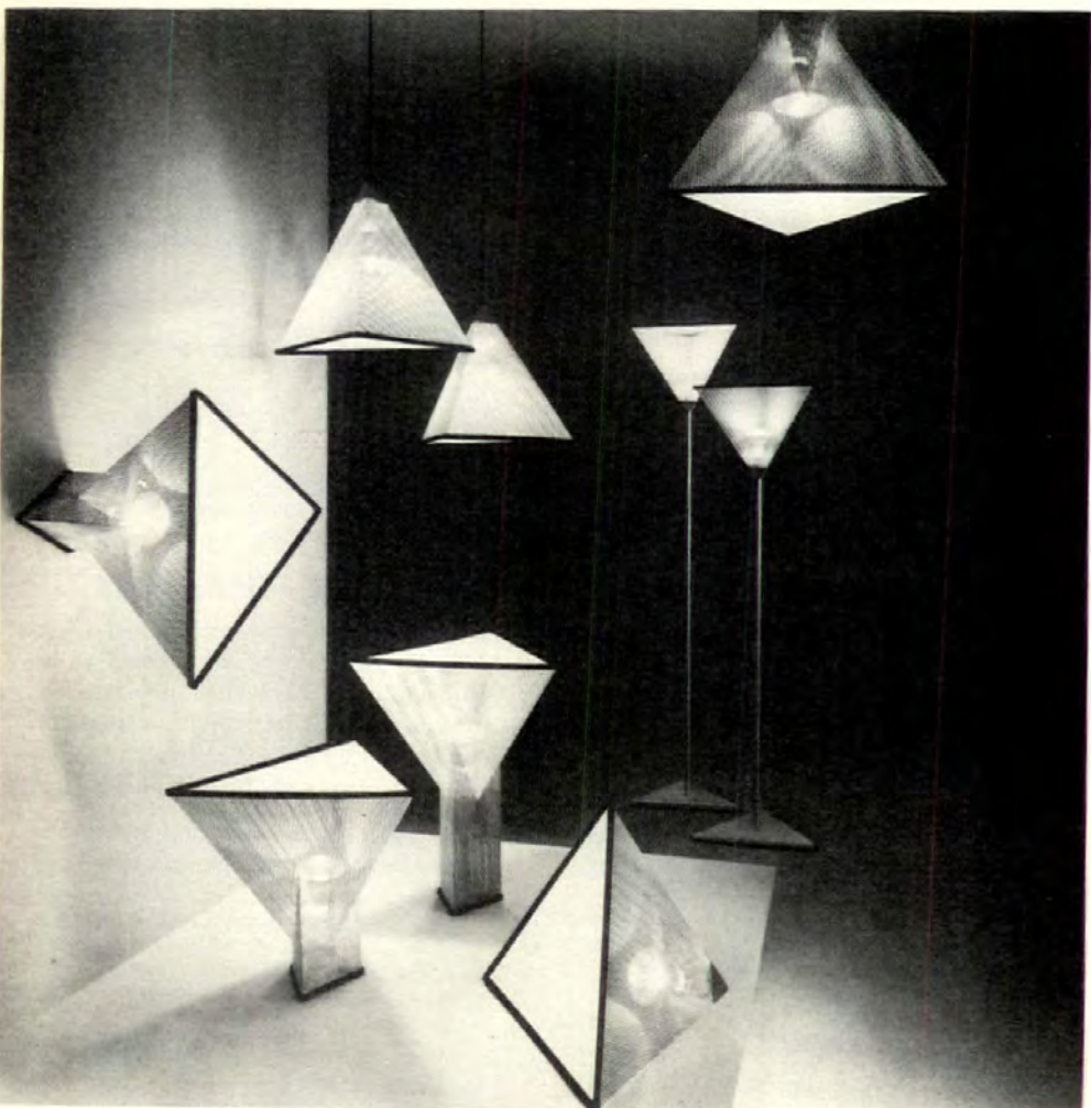
Lighting system, "Trianglo," includes floor, wall, ceiling and table models. Geometric fixtures are constructed of perforated color-baked metal sheeting with all exposed edges trimmed in black rubber. Basic shade is an 18" triangle; floor lamps are 64" and 84" high. Koch + Lowy, Long Island City, N.Y. CIRCLE 214 ON READER SERVICE CARD
