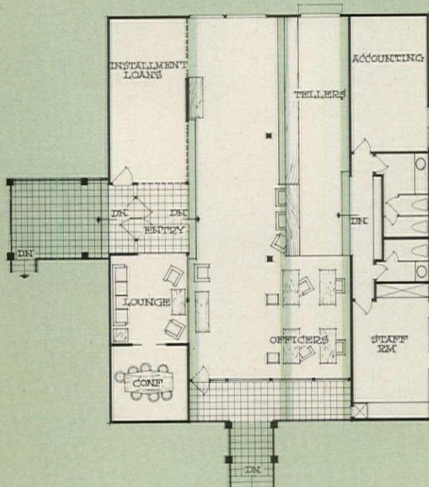
Rectangular plan of bank is made of four modules. Center units are shorter to leave room for deck.
