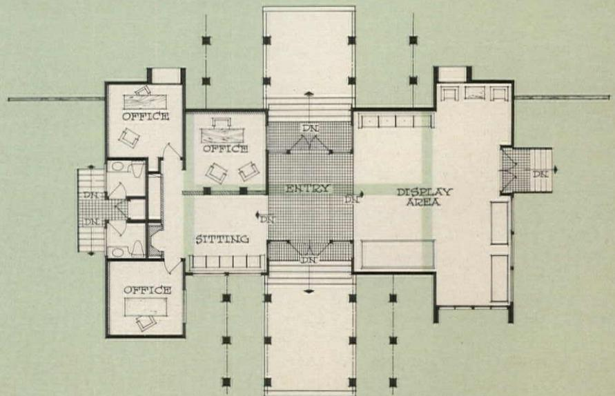
H-shaped plan is made of four modules. Open area at right is sales office's display room.
