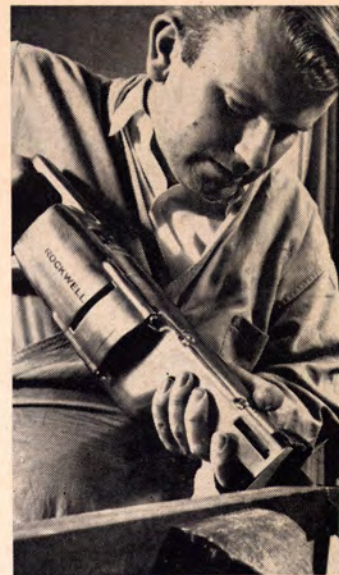
Bayonet saw with orbital blade action cuts through 2½" wood, ¾" aluminum, and ¼" steel. The base—17 sq. in.—tilts 45° left or right for bevel cutting. Industrial-rated 3-amp motor produces 3,500 strokes per minute. Rockwell, Pittsburgh.
