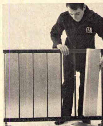
Snap-together radiator for hot water or steam consists of aluminum radiating elements that fit into a steel-tube frame. The unit is only 2" thick, and lightweight, and its small water capacity minimizes scale deposits. Feal, Milan, Italy. Circle 318 on Reader Service card
