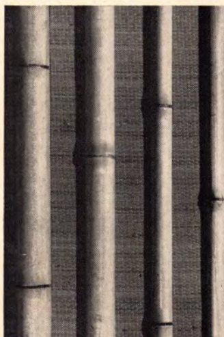
Bamboo molding is made of half-round wood with darkened knuckles at 9" intervals. Advantage over real bamboo: It can be mitered. The trim comes in 3/4", 1 1/4", and 1 1/2" widths in lengths up to 8'. Federal Millwork, Ft. Lauderdale.
