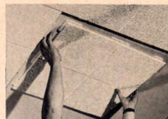
Ceiling tiles molded from polystyrene have a white pebble-textured surface. The 24"x24" squares are prescored to give the appearance of 12"-square tiles. Interlocking flanges facilitate alignment. U.S. Mineral Prods., Stanhope, N.J.
