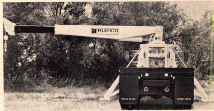
Truck-mounted crane rotates 360° in either direction, elevates to 90°, and lifts up to 16,000 lbs. Two self-centering levers control all movements of the hydraulic, telescoping boom. Also: a 10,000-lb.-capacity model. Alenco, Bryan, Tex. Circle 242 on Reader Service card
