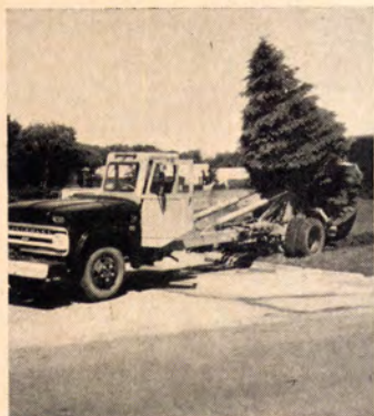
Truck-mounted tree mover has two hydraulically operated cutting cups that scoop out a root ball in minutes. The tree is hoisted hydraulically and laid prone for transport. Capacity: trees up to 8" in diameter. Vermeer, Pella, Iowa. Circle 241 on Reader Service card
