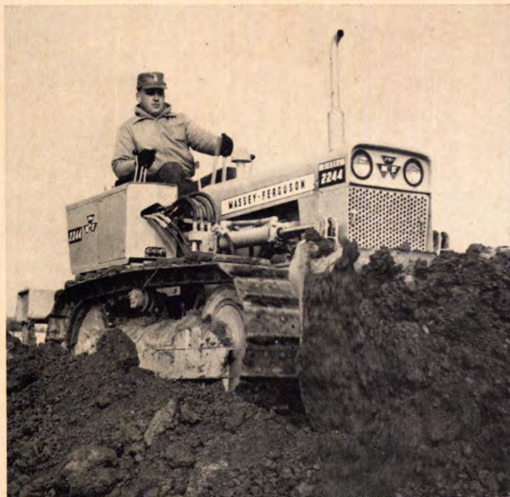
Crawler tractor with 44 hp. diesel engine offers long-track design for easier maneuvering. Tension on five-roller track frame is adjusted hydraulically in an estimated two minutes. Track roller guards are standard. Massey-Ferguson, Detroit. Circle 238 on Reader Service card
