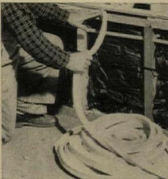
**Insulation strip**, designed to cut labor cost of caulking around doors and windows, is simply pushed between studs or sills and door or window frame. Bonded cellulose fiber strip is  $\frac{3}{4}$ " x  $1\frac{1}{4}$ ", comes in 50' rolls. Wood Conversion Co., St. Louis.
