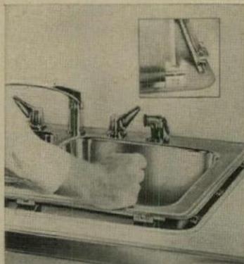
**Stainless-steel sink** in maker's low-cost line now has a factory-mounted rimming-locking device, needs neither separate frame nor rim. Spring clamps simply snap sink to retaining strips nailed along the inside edge of the counter cutout. Elkay, Broadview, Ill. *For details, check No. 18 on p. 155*
