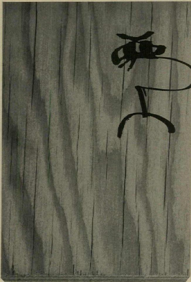
Both of the above panels—CreZon Overlaid Plywood and regular plywood—have undergone a grueling 8-day torture test designed to demonstrate resistance to weathering. For four cycles, 192 consecutive hours, they were alternately boiled, steamed, frozen and baked dry—the equivalent of years of weather exposure.
