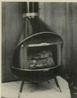
**Open hearth fireplace**, called the Firemite, incorporates principles of circulating fireplace form. Elements include heavy steel base, self-cleaning grates, inner circulating form, outer hood, fire screens, and insulated flue. Air circulating between shell and hood cools hood while warming the room. Finished in black or color.
