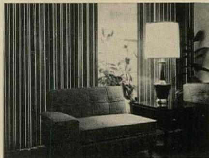
**Accordion divider** is made of thin mahogany panels laminated to two layers of opaque vinyl. Forestfold is punched along the bound top edge with metal eyelets and can be furnished with glides and track. Standard heights are 6'8", 7', and 8' in any width to 30'. Price is competitive with quality drapery.
