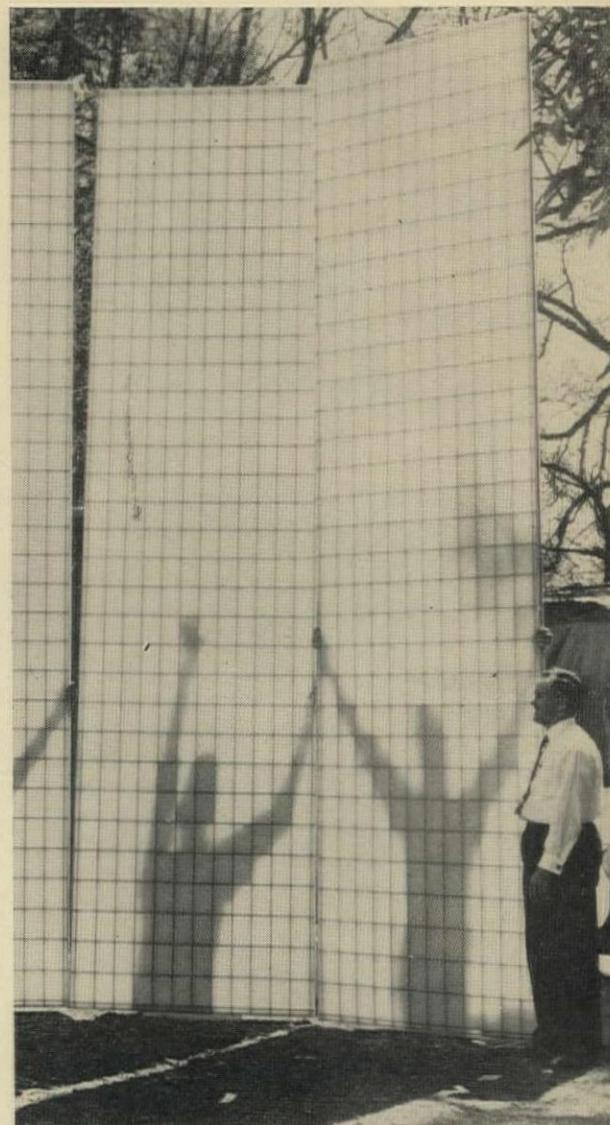
**New sandwich panel** consists of two translucent fiberglass-reinforced skins laminated to a 4"x6" grid of plastic fiber strips. Elimination of through metal gives the panel a U value of only .35. Panels are available in stock and custom sizes to 4'x20' and thicknesses of 1/2" to 3". Builder price in large lots is less than \$3 a sq ft.
