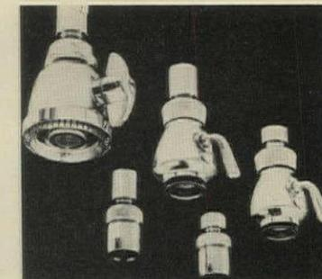
**Showerhead line** with built-in automatic controls is new from Dole Valve. Automatic valve opens or closes with changing pressure to hold a 3-gpm flow.
