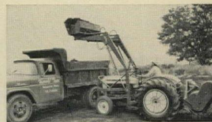
**FRONT-END LOADER** skims and loads topsoil
