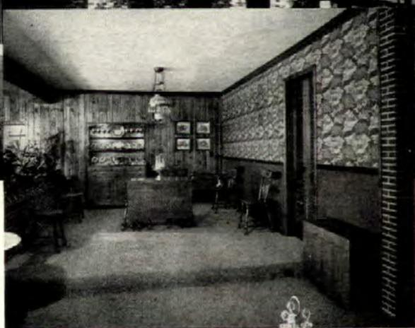
AT LOWER RIGHT in above photograph is one of the units which are used throughout the house. Revere Copper Water Tube carries hot water to the units in winter and cool water in the summer. Fans in the cabinets then circulate the hot or cool air, as the case may be, throughout the rooms.
