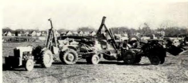
**Back-hoe** (left) and **high-lift** (center) Schmitt added to combination of two (right) when he built 50 houses a year. As used machines, back-hoe cost \$4,000, high-lift \$800. See questions No. 17; 22.
