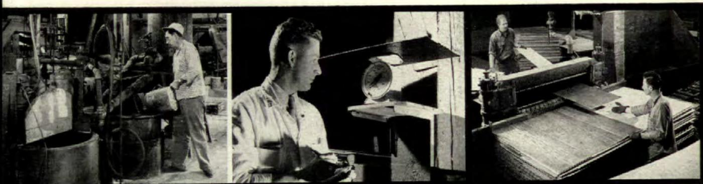
**4** AT THE GLUE MIXER, check for complete adherence to glue manufacturer's mixing directions. Special formulae developed by million dollar glue company research programs. Before any glue is approved for use in plywood, the manufacturer must submit products for performance testing under factory conditions.
