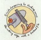
Finish by stroking down and across the cutting edge with an eight-inch bastard file. Match the angle of the manufacturer's bevel. Sharpen fine cutting tools, such as knives, with a diamond hone.
