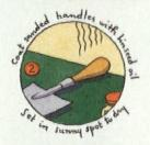
Wipe handles with a damp cloth, then coat with boiled linseed oil. Set in a sunny, warm spot to dry.
