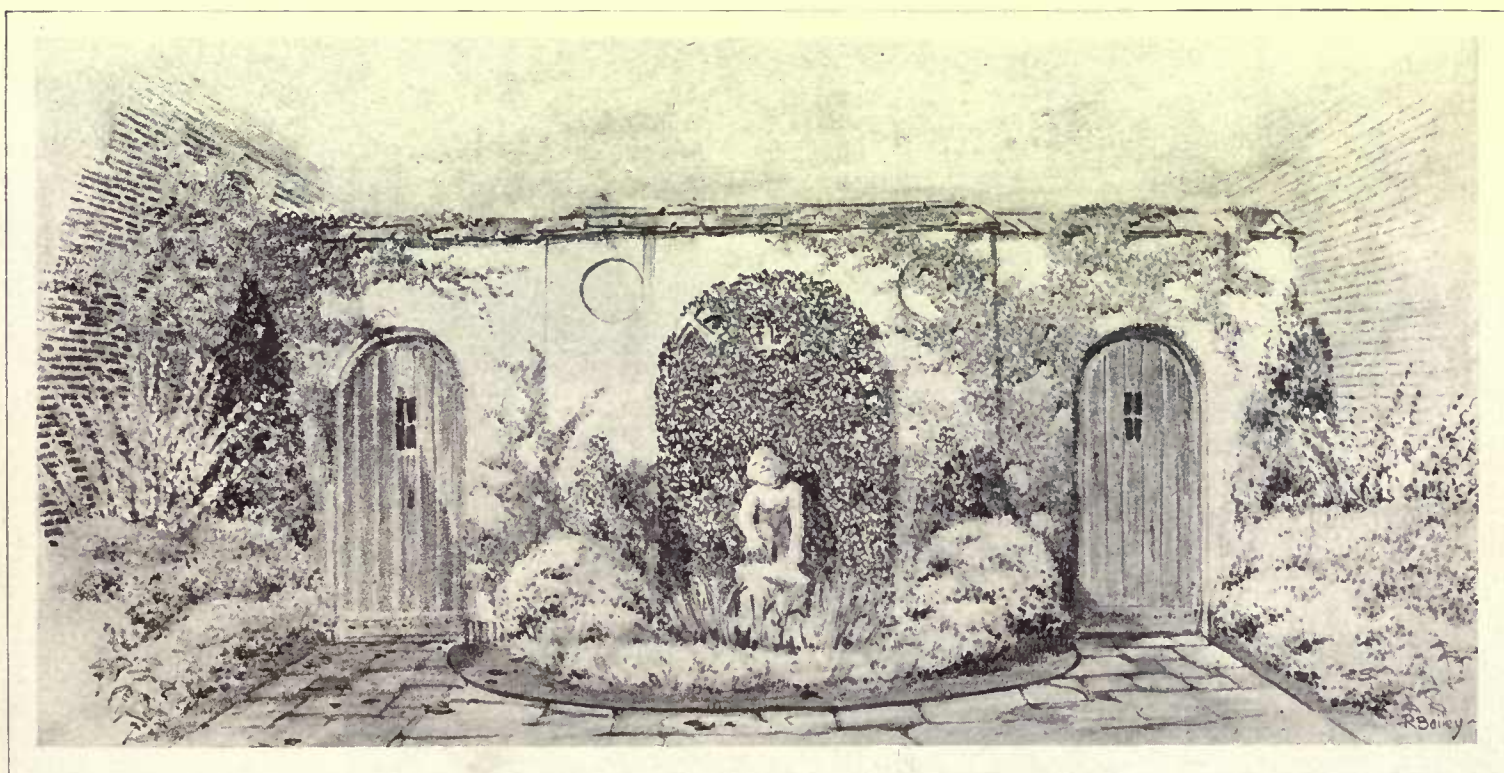
A wall of this kind, used to separate the garden and the laundry yard, may be made of hollow tile and stuccoed. The coping and
