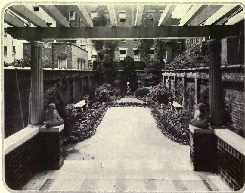
The terrace at the rear of the house, treated as a pergola, makes the transition between the living room and the backyard garden which extends to the end of the plot. To heighten the wall at the rear and make it a more effective screen a lattice has been erected on it
