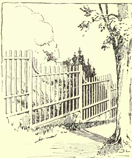
An effective solution of the hillside fence whose stepped sections are joined by a bit of curved rail
