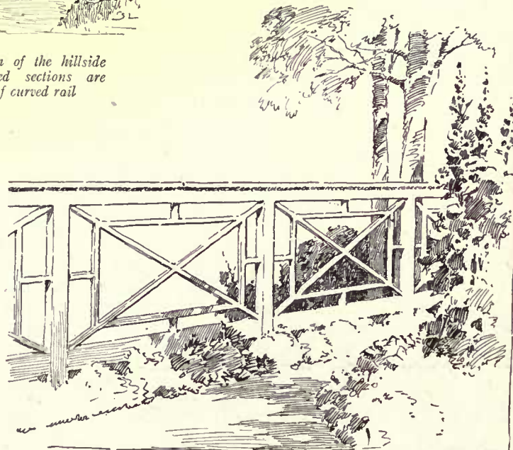
When a fence need not be a complete barrier against small animals more latitude may be allowed, as here, in the decorative arrangement of the braces
