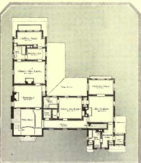
Based on an L, the plans of the Light house show on one side a long living room with solarium, and dining room and service on the other, a loggia connecting them. On the second floor a long corridor between stair hall and service stairs is a feature
