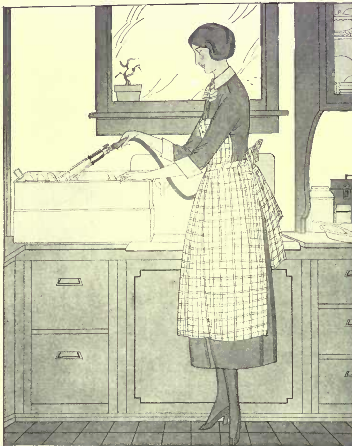
The simplest form of dishwasher consists of a stream of hot water from a washing nozzle attached to the hot water faucet and directed by hand. The nozzle contains a soap mixer, operated by a thumb lever, so that soapy water is delivered for washing and clear for rinsing. The dish pan has a splash board. Courtesy of the Torrent Utilities Co.
