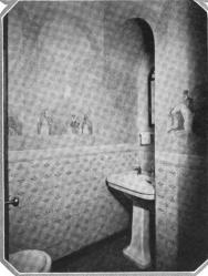
In one of the baths the plaster walls are painted in scenic panels above a vainscot of blue picture tiles which are also painted on. The woodwork is finished in deep blue
