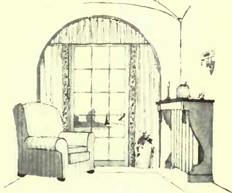
In an enclosed porch a shelf can be built above the radiators, supported by side brackets. The top may be marbleized
