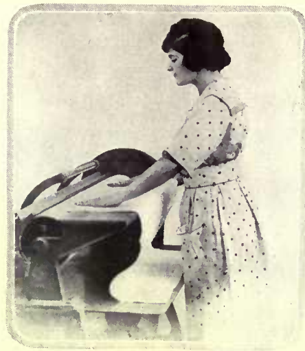
Laying a flat piece in an ironing machine is made easy by the feed-board. Courtesy of the Hurley Manufacturing Co.
