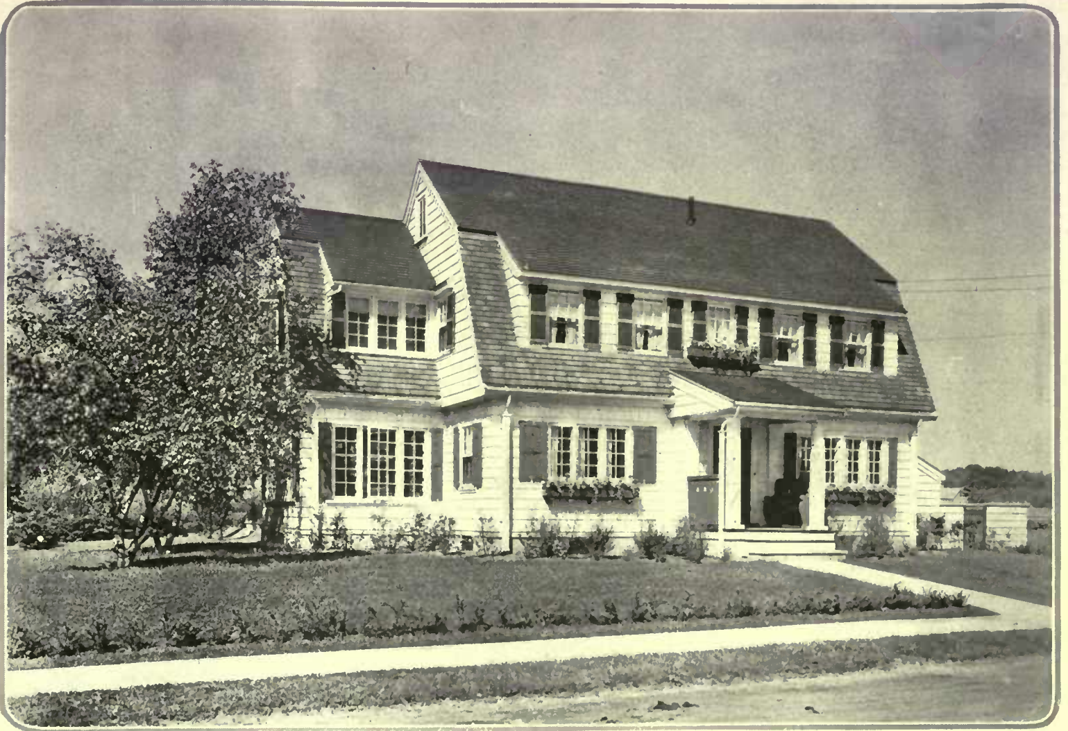
The gambrel roof type is a popular design because it makes a roomy house. Its architecture is intimate, informal, and it suits most settings. In this interpretation a wing, in the style of the main house, is added at one end. The windows are grouped in a pleasant fashion, with shutters to finish them and to give a note of contrasting color to the white shingled walls and woodwork. The entrance is pronounced by a portico with high-back settles on each side
