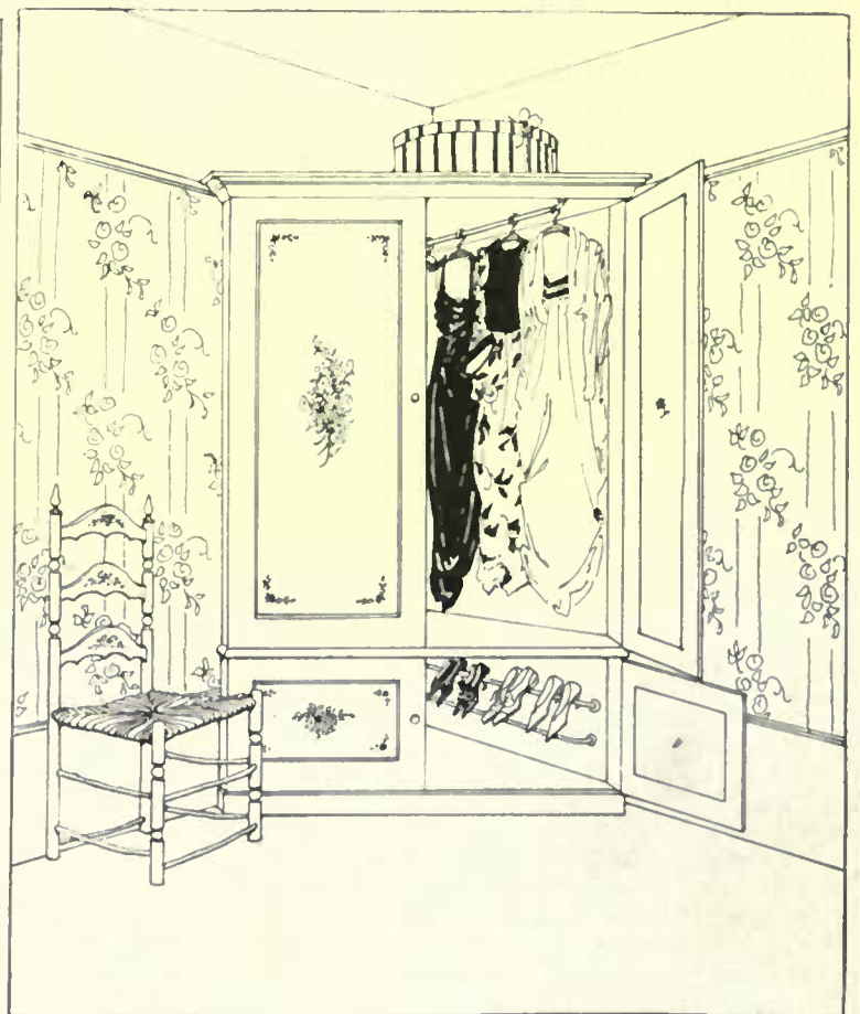
The built-in corner cupboard can be made from an inexpensive stock wardrobe set at an angle to the wall and built up behind. Shoe rods go in the compartment beneath and the clothes above. Designed by Agnes Foster Wright
