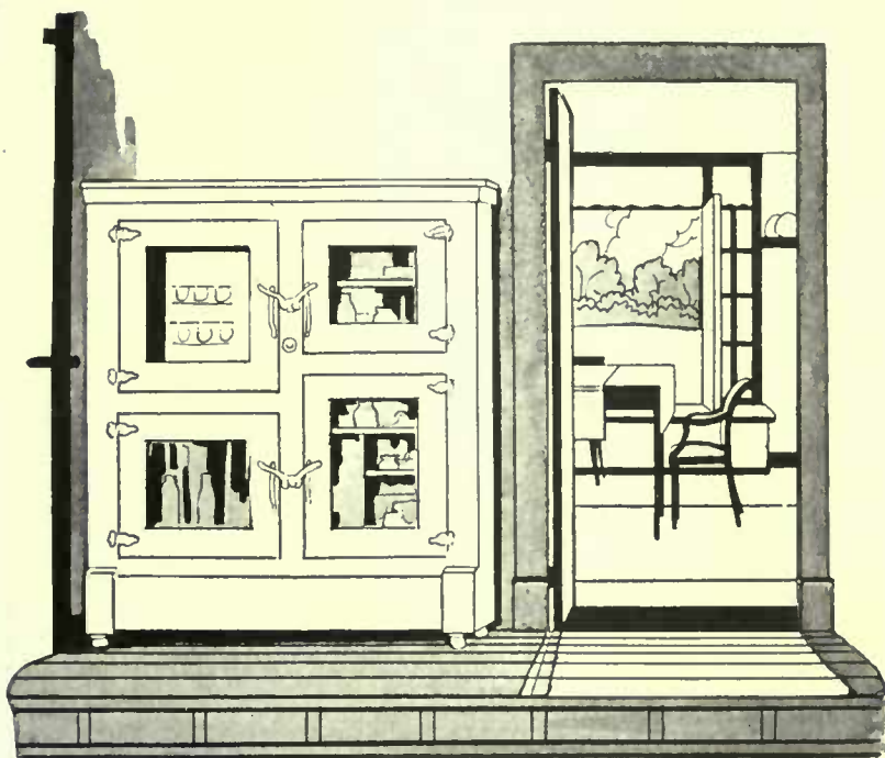
In several of the systems the machinery is placed in a compartment at the bottom of the refrigerator with the coil box and ice making trays in a section above. Where the machinery is so installed it must work silently. Courtesy of the Frigidaire Corporation
