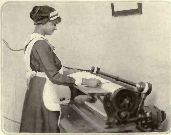
For ironing flat work comes an electric iron with motor. Courtesy of the Edison Co.
