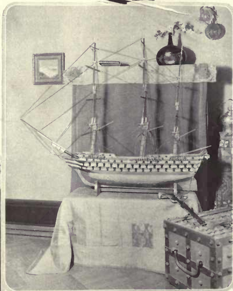
The early American ship of the line was a boat with beautifully complicated rigging and carried four gun decks. This model, from the Harrison Cady collection, is a picturesque and reliable example
