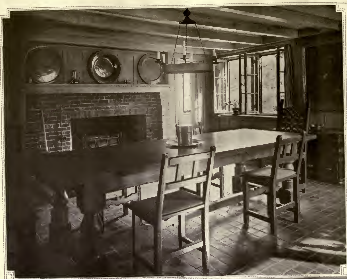
The walls are plain grayed cypress boarded and batted. Simple window openings and casements establish the cottage atmosphere, which is further accentuated by the antique English oak furniture
