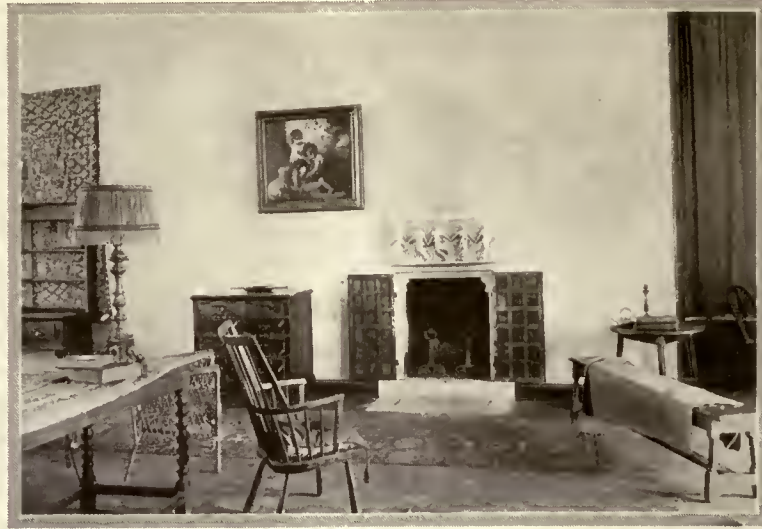
Martin In this gated fireplace is the germ of a suggestion to use folding screens attached to each side of the fireplace or wrought iron gates to arrest the sparks. Myron Hunt, architect
