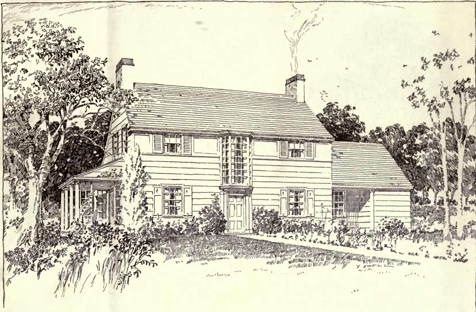
On the front a long bow window, extending the height of the second story, is the unusual departure from the Colonial design which distinguishes the house. It affords a tight hall which can serve as sitting room or sewing corner. Plain panels are used instead of shingles on the upper spaces beneath the eaves. The little service porch is a convenient feature
