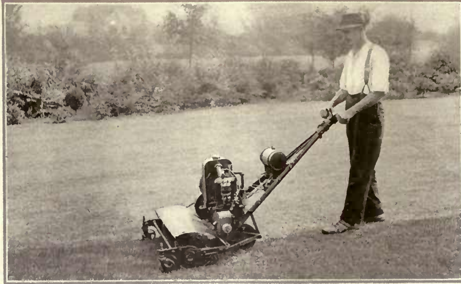
Labor is lessened by a power mower that can be used for both trimming around trees and shrubbery and straightaway work
