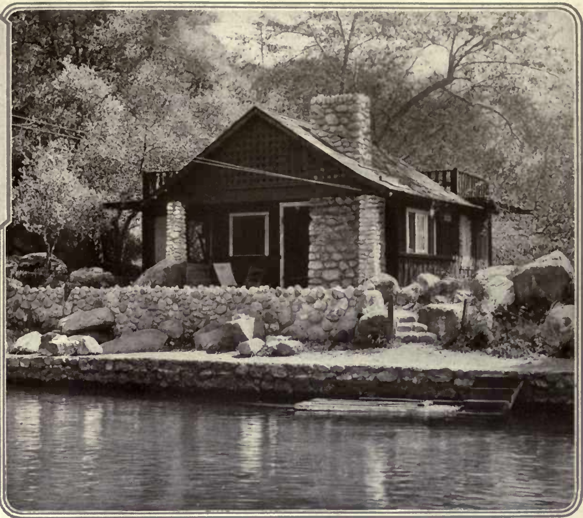
An interesting mountain camp is built of 3" planking laid in cement to simulate logs. These are oiled and stained a rich brown, the shingled roof is painted a soft green and the trim white. The living room and dining room have fine woodwork flooring stained olive green, and tinted plaster walls. The kitchen is finished in white enamel. The approximate cost was $500. H. H. Whiteley, architect
