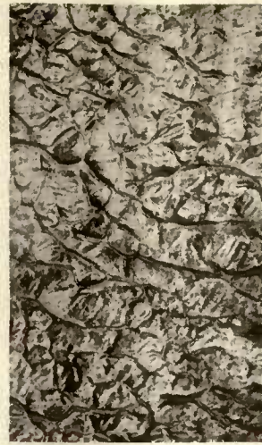
Wrinkle mottle is one of the most curious forms of this figure. The example here is of mahogany
