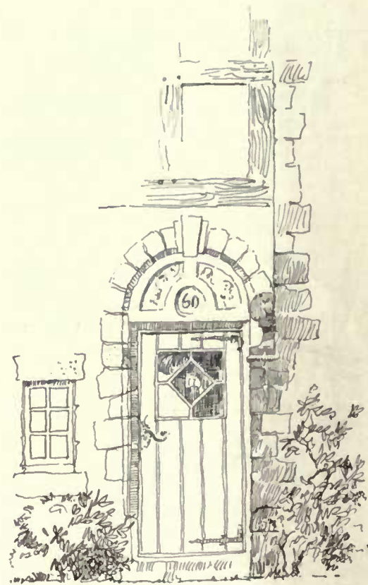
Above the entrance door would be a recessed plaster tympanum with a stone facing. The door itself is made of heavy oak planks fitted with wrought iron hardware. This detail shows the treatment of the exposed stone or brick corners
