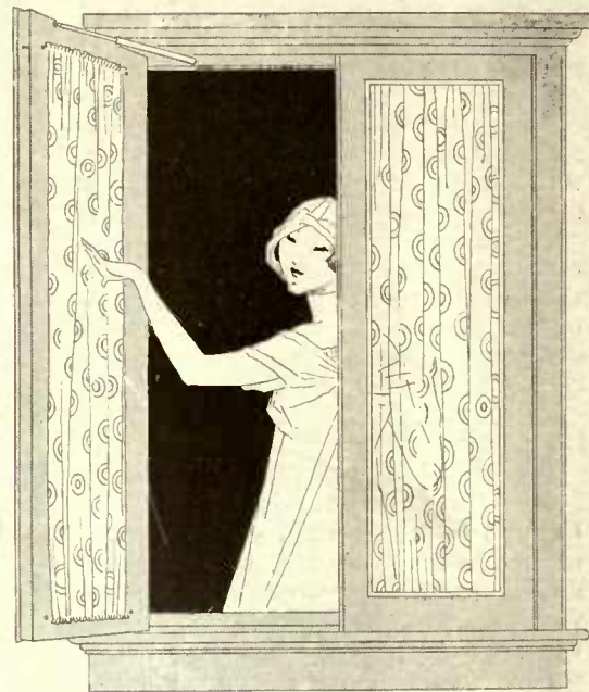
You push open the casement and it stays open. Such desirable behavior is due to a collapsible catch at the top
