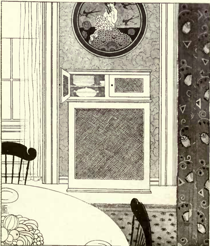
Enclose the dining-room radiator in a box with rattan panels and build shelves above; a serviceable warming closet has been made
