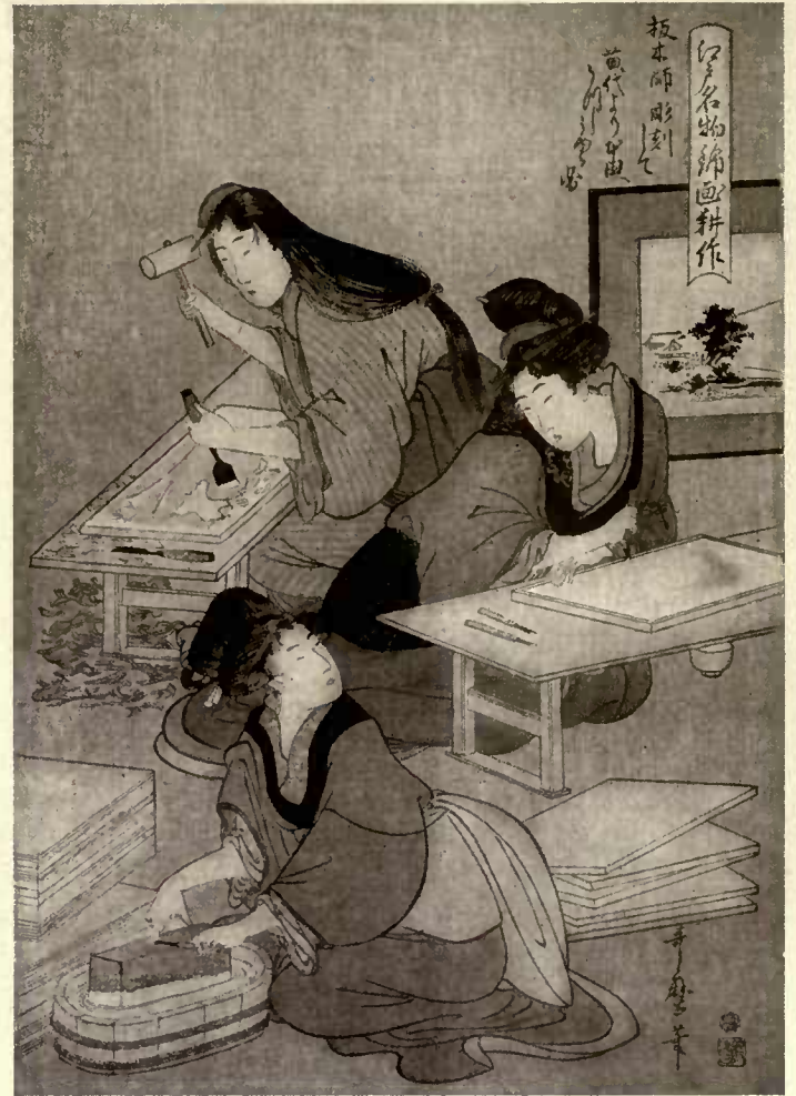
The color print process, by Utamaro (1753-1806). The figure in the foreground sharpens the engraving knife, the other two work on the outline and chisel the block
