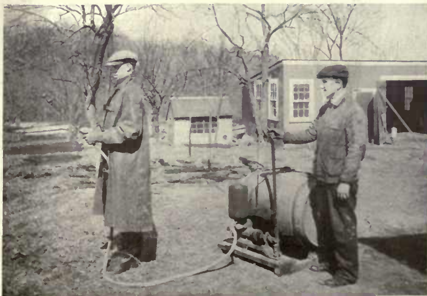
The barrel type of apparatus can be mounted on runners for winter use or on wheels for moving about when the ground is bare
