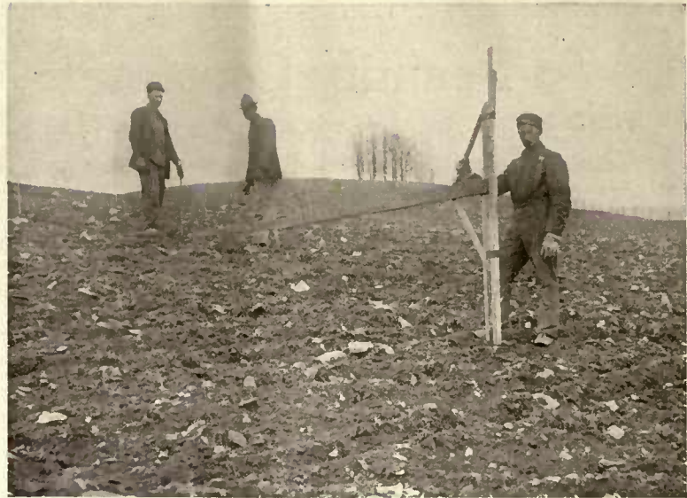
In setting the trees on the hillsides a homemade "leveler" was used to determine their exact locations
