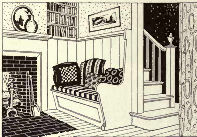
Figure 1—An enclosure forming the back of a bench next to the fireplace utilizes the corner and screens the stairs. An upholstered seat such as this adds to the comfort. Use the bottom for a woodbox
