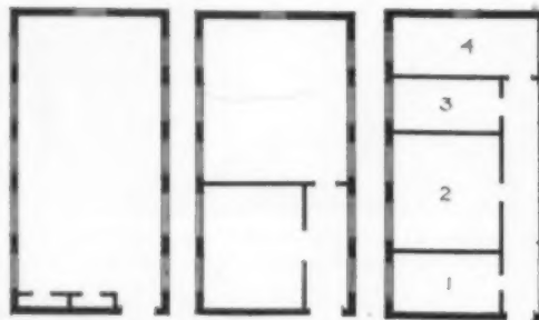
Plan showing arrangement and division of sleeping porch by means of sliding panels
