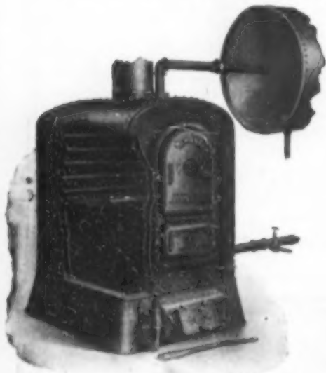
A small coal fire is started on the lower grates. The by-pass at the back (a patented feature of the Kewanee) prevents the wet and damp garbage from smothering the fire. The garbage is quickly dried and burns without odor. The garbage grates contain water and the entire chamber is surrounded by water which heats water hot in abundance.
