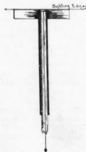
A T-square mounted on a stake with a plumb-line attached serves as a sighting instrument in determining contours
