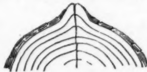
A cross-section showing a typical frost crack
