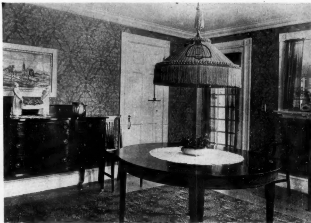
The lines show the lighting arrangement inside the silk shade. The globe should be of dense depolished opal; the shade lowered as indicated. The upper arrow shows position of a small dimming device
