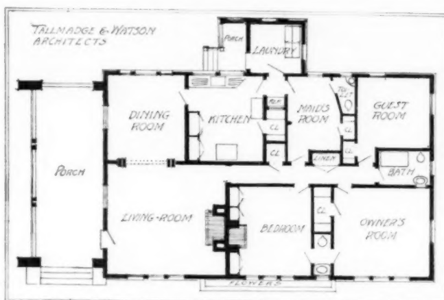
For a narrow lot it is more difficult to work out a satisfactory plan. If one is willing to dispense with an entrance hall this is an excellent arrangement
