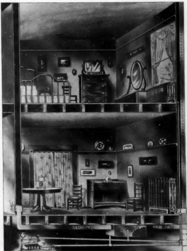
There are three different methods of radiation: The direct, the semi-direct and the indirect.
