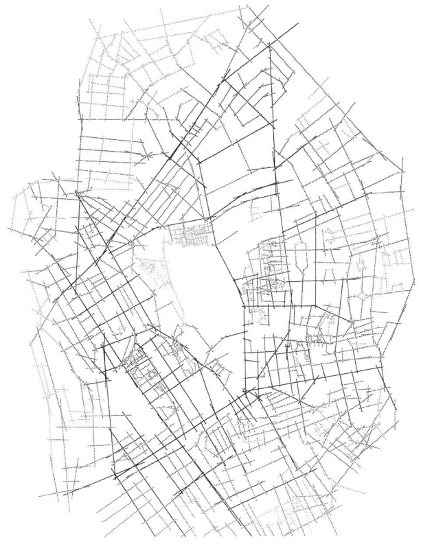
figure 27 Axial map of figure 26 analyzed in terms of its distribution of integration, with the most integrating lines shown darkest, graded towards the least integrating shown lightest. Since integration predicts natural movement, one can think of the blackness (i.e. dot density) of the line as predicting the amount of movement down that line.
