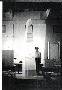
Our first roof experiment in our studio. Folded corrugated plastic—a failure.
