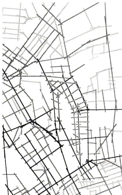
figure 38 Final scheme for King's Cross masterplan analyzed in urban context to show how it affects the pattern of integration.
