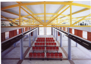
Interior: Industrial-type materials such as concrete floors, steel trusses and beams, and metal doors, gates and roll-up shutters combine with natural light and ventilation to create a comfortable waiting room. The color scheme adds interest and reflects local pride.
