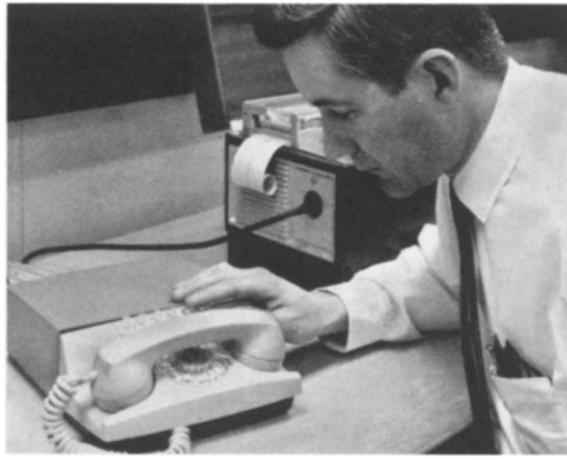
Telephone adapter for transmission of electro-cardiograms of patient's pulse directly to doctor.
