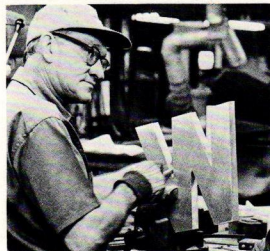
Finishing sawed metal forms.
