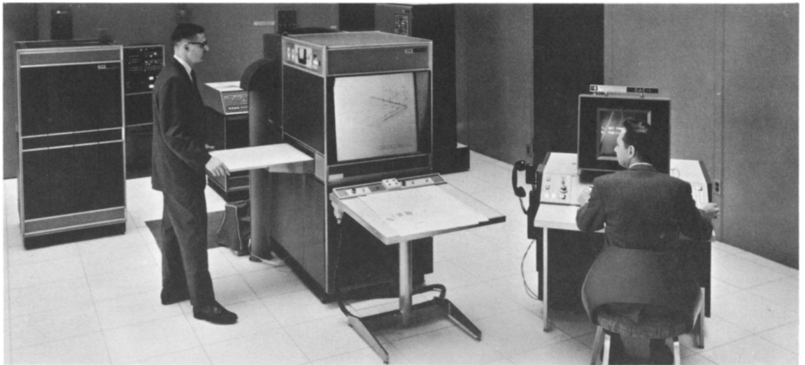
The DAC-1 system showing the Image Processor which provides input and output in graphical form (center) and the Graphic Console which contains a cathode ray tube, card reader, keyboard and program function switches and indicator lights (right).
