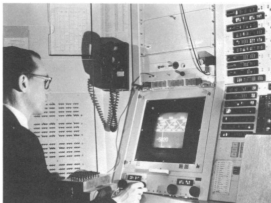
Dr. Ivan E. Sutherland working on a Sketchpad display tube mounted on the console of M.I.T.'s Lincoln Laboratory TX-2 computer. Push buttons used to control specific drawing functions are on the box in front of him. Size and position of the part of the picture seen on the display tube is regulated by means of the four black knobs below the screen.
