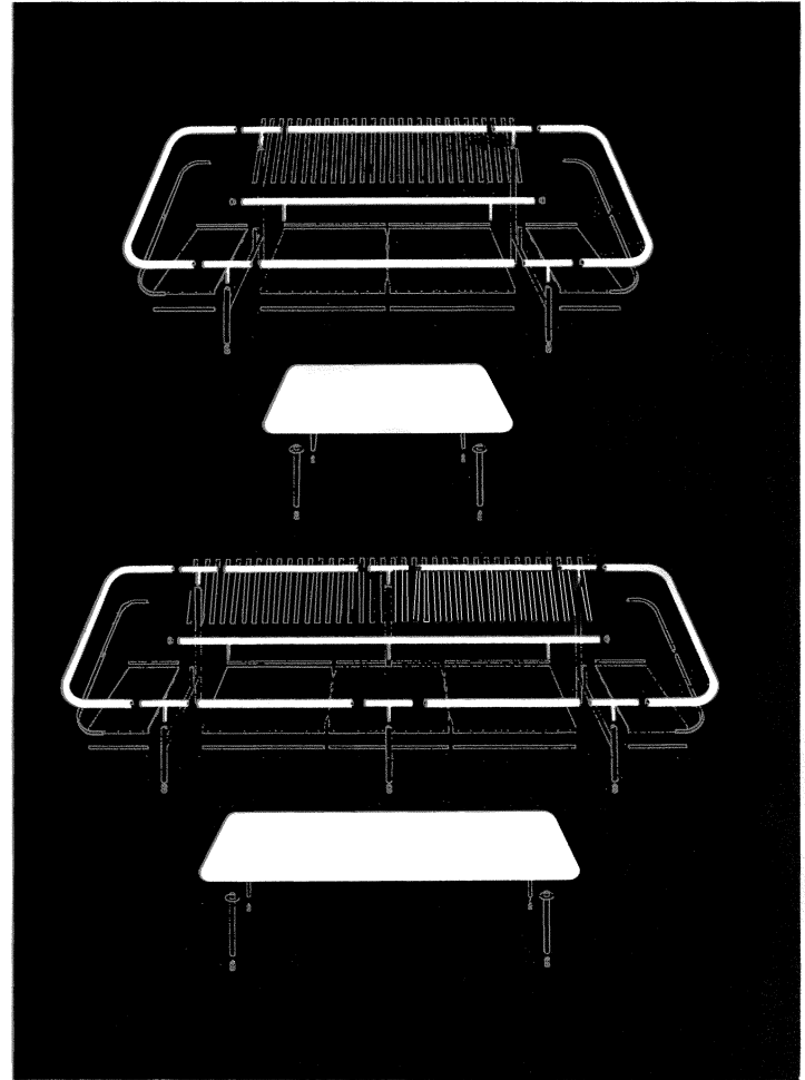
Informative communication: Exploded drawing of sling sofa designed by George Nelson and Co., Inc. (Manufactured by Herman Miller, Inc.)
