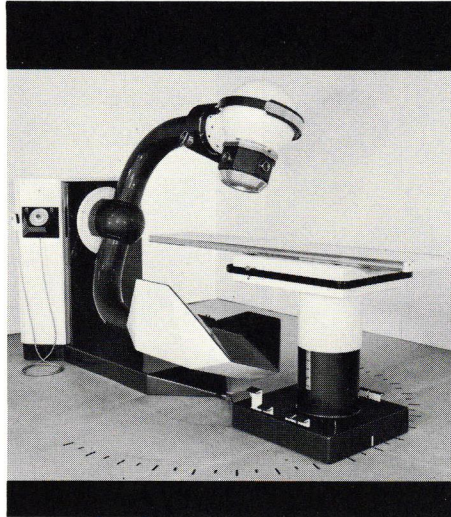
49. Telecuring medical equipment with radioactive cobalt 60. Design: Manufacturer's team, Philips Electrical Works.
