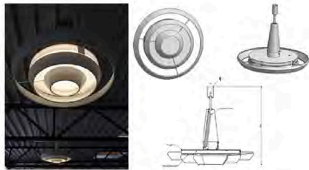
Figure 3 – Integration of LED technology in the original Regent lamps. © photo: Roberta Grignolo; drawing: Regent Lighting.
