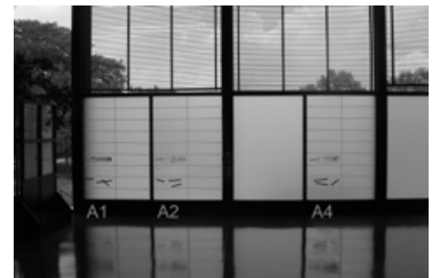
Fig. 8. Mies van der Rohe, Crown Hall, Chicago IL 2004, Krueck+Sexton, Mock-up sample of various materials on glass to test seal
