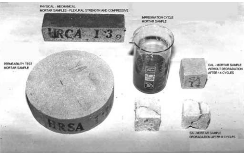
Figure 3. Left: Ornamental Mortar, Durability Test. RILEM 25 PEM. Samples and System. Right: Ornamental Mortar, Physical-Mechanical Test Results.
