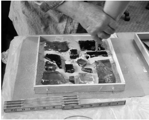
Figure 4. Epoxy is being poured around the hammer-cut and faceted dalles and aggregate will be added on top as the finish surface; no other materials are involved in producing these panes. Photo: F. Chou
