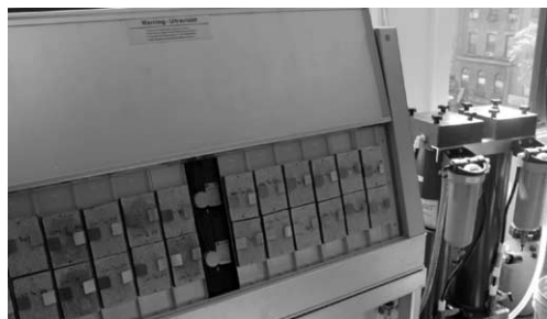
Figure 3. QUV-Spray weathering machine with mounted samples. Photo: Amanda Thomas Trienens.
