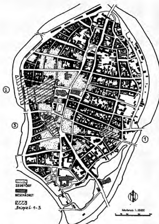
Fig. 2 – Plan of the historic center of Lübeck with the damaged areas resulting from the bombing raids from 28./29. March 1942 zerstört = totally destroyed beschädigt = partially destroyed areas Examples discussed in this paper: 1- Krähenstrasse 2- Merchants Quarter 3- Schmiedestrasse Source: (Beyme: 1992)
