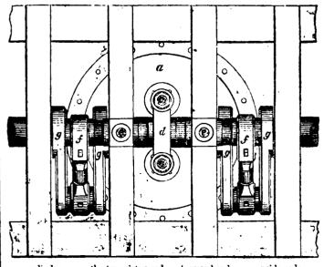
a, cylinder. c, c, the two piston rods. d, cross head. e, e, guide rods. f, f, connecting rods. g, g, g, g, g, c, cranks.
