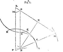
Let A B and C D, (fig. 1) be the two given curves (say of 130 chains radius), and let it be required to unite them by a third curve of less radius, tangent to A B on its concave, and to C D on its convex side.
