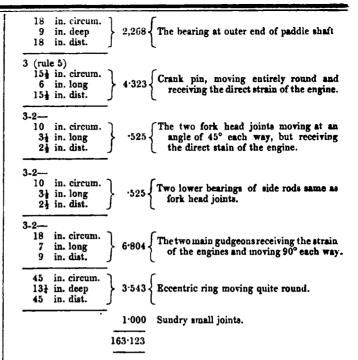
Therefore, if it be assumed that the total quantity of friction in a steam engine is as 163-123, then will the relative quantity of friction in the several parts be nearly as is represented by the numbers in the preceding table.
