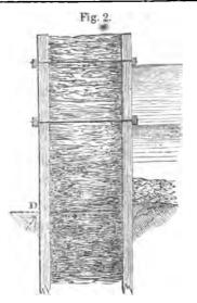
Put s for the mean weight in lbs. of a cubic foot of the materials in the dam, b for its height in feet, d for its width in feet, and c for the depth of high water in feet. We then have b d e equal the weight of one foot in lenght. It is evident that the dam fails only when the force of the water is able to turn it round the point D, and as the weight b ds acts at the distance  $\frac{d}{2}$  from D in the figure its force is pro-
