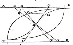
parallel to E'H, the bisection of the interval between these will give the horizontal projection of the joint. Similarly, the side and end projections are modifications of those belonging to the circular arch:they are fully investigated in the appendix.
