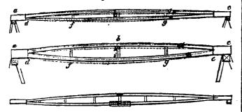
He then took pieces of fir 50 in. long, 2 in. deep, and 1 in. wides one was left solid, two others were slit so as to make the upper part It inches deep, and the under 2 in., one piece having the slit half the depth of the beam apart, the other 2 of the depth apart. See fig. 2. Is will be perceived that the principle of this system consists in the
