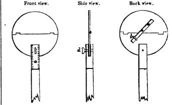
It consists of a disc of tin about six inches in diameter, which for convenience in carrying may be joined across the middle as shown in the accompanying sketch; its open position being secured by a little bar A to be turned into the latch B. An iron ring or socket C is screwed on the top of the pole and receives the disc in a slit while the screw D secures it. It is almost needless to remark that the disc should be painted white on both sides.
