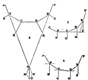
Assuming the system of points A, B, C, &c. fig. 6, to be in equilibrium, we shall now imagine the connecting lines to become perfectly rigid. It is evident that this supposition will not affect the equilibrium, as it does not involve the addition or abstraction of *force*, the only agent by which equilibrium is preserved or destroyed. If then the system was in equilibrium before, it will remain so now, and we have consequently a rigid body acted upon by the forces V, P, Q, R,
