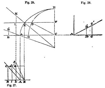
Let A B C in the annexed diagram, called fig. 27, represent the plan of the acute quoin of the arch, then when the point A may have ascended to the altitude signified by  $\tau$ , let us suppose it to be perpendicularly over the point E, fig. 27. Let us also suppose A C fig. 27
