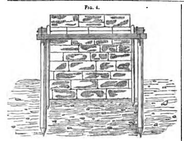
as possible by means of dredging with the common bag and spoon apparatus, the stones were brough to the place in hoats, and lowered by a crane, in such a way that as soon as each stone was placed in its proper position the *lewis* could be withdrawn without difficulty.
