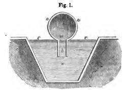
If such a tube is haid all along upon the ground, with the iron channel immersed in a channel of water, up to m, and a piston or box made to fit it loosely, and pass through it upon wheels or rollers, this box, driven through the tube by the air forced into it, may give motion to a carriage without, by a communication through the channel and the water.
