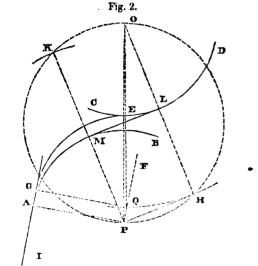
Let A B, C D (fig. 2) be the given curves, the former being tangent to the straight line I A at the point A. To draw a common tangent to the two given curves.
