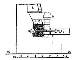
p six pigs of iron ballast, each 56 lbs. to prevent the brickwork separating by the heat, h Hood. G. L. Ground Lane.
