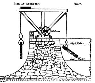
The author next proceeds to describe an economical method of building the foundations of a pier as practised by Mr. Telford at Inverness, to avoid the expence of erecting a coffer dam. This is well deserving of notice on account of its simplicity, particularly the part explaining the "lewis."
