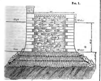
in front, with dry stone hearting of squared scapple dressed rubble inside, and in this way was carried up to the full height required.
