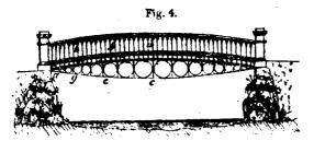
The application of this system to roofs and floors is extremely economical and useful, and by simple modifications serves for the covering of large spaces without any intermediate point of support, and presents this further advantage, that from its vertical pressure it requires no other support than walls of moderate thickness.
