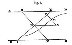
Let AB, CD, represent the two abutments, HN the crown line, GF and PN the horizontal projections of two of the lines of pressure.
