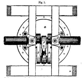
a, cylinder. c, c, c, c, the four piston rods. id, cross head. e, e, guide rods f, connecting rod. g g, crank.
