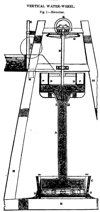
THE accompanying engravings represent a vertical water-wheel, upon the principle of Barker's mill, which I erected at the ironworks of the United Mexican Mining Association at Durango, in Mexico, in 1832, for the purpose of driving a circular saw; it was desirable to produce a rapid movement without the intervention of gearing, and this not being possible by means of the breast wheel, which was, besides, fully loaded with the blast machinery, it occurred
