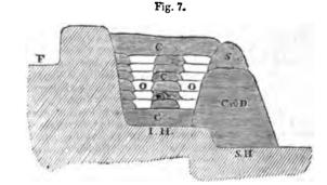
REFERENCES. -I. H. Iron Hearth. -S. H. Slag Hearth. -C. and D. Charcoal and Dust. -S. Slag. -C. Charcoal. -O. Ore. -F. Floor.
