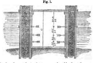
each other, the next best point to secure is evidently at the centre of pressure of the whole depth of water, or using the same notation as before at  $\frac{1}{2}$  c from the bottom. If more stays are necessary, the most
