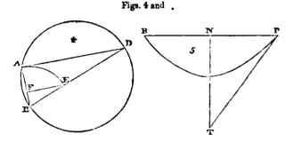
That is to say, the forces applied at the several angles of the polygon are proportional to the cosines of the halves of those angles. Let us now suppose that the lines A B and B C are equal to each other. Through the points A, B, C, fig. 4, describe the circle A B CD, draw the diameter BD, the arc A E, and E F at right angles to A B. Then B D bisects the  $\angle A$  B C, and because B A D is a right angle (Euc. p. 31. b. 3):--
